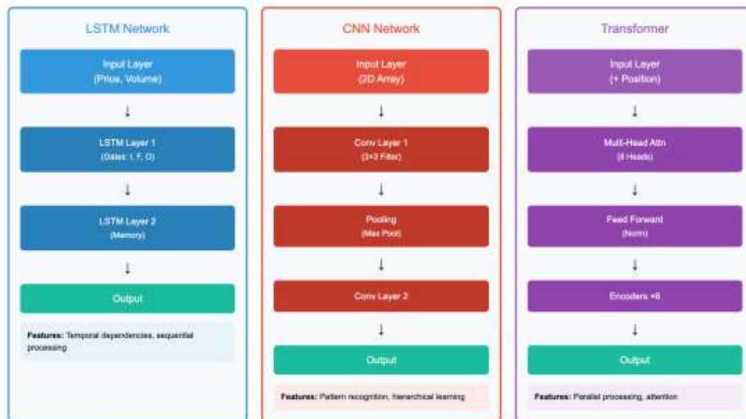
Figure 1 Caption: Architecture comparison of three neural network types applied to financial time series forecasting. The LSTM network processes sequences through memory cells with gating mechanisms. CNN extracts local patterns through convolutional filters and pooling operations. Transformer uses multi-head attention to capture dependencies across all time steps in parallel. Each architecture processes historical S&P 500 index data (2020-2024) to predict future prices.
